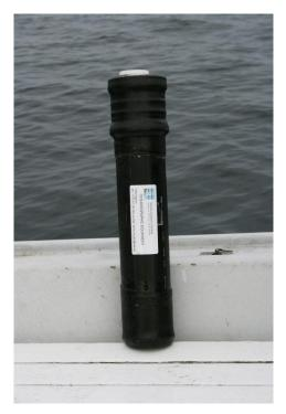
Figure 33 Autonomous drifter buoy developed by Tallinn University of Technology
