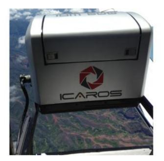
Figure 11 Multispectral sensing system - the Icaros IDM600 sensor [16]
