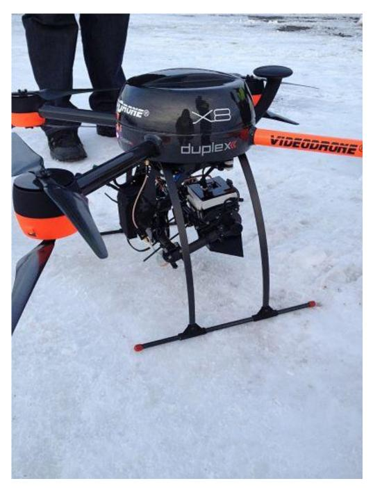
Figure 22 Thermal infrared camera attached to the drone.
