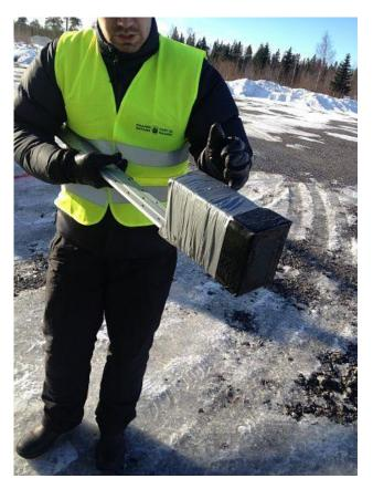
Figure 26 Hyperspectral camera inside the insulation box.
