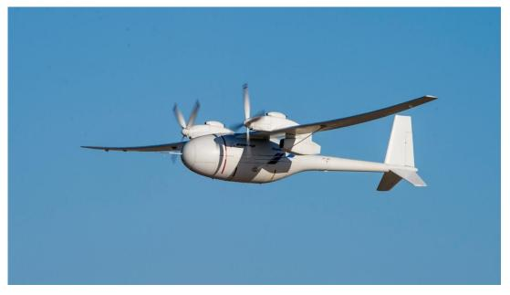
Figure 2 High Altitude/Long Endurance (HALE) UAV - Boeing Phantom Eye [3]
