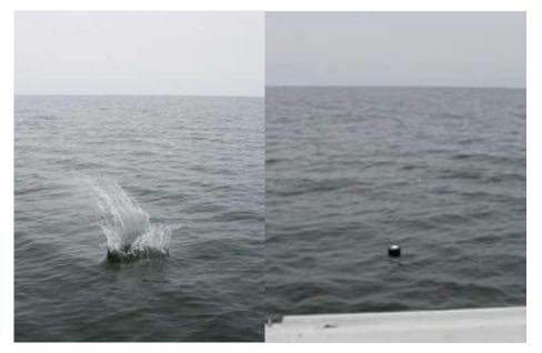
Figure 35 Deploying the drifter from the boat (left panel) and drifter in working position (right panel)
