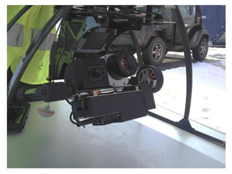
Figure 2 Infrared camera with the larger lens and smaller device for object detection.
