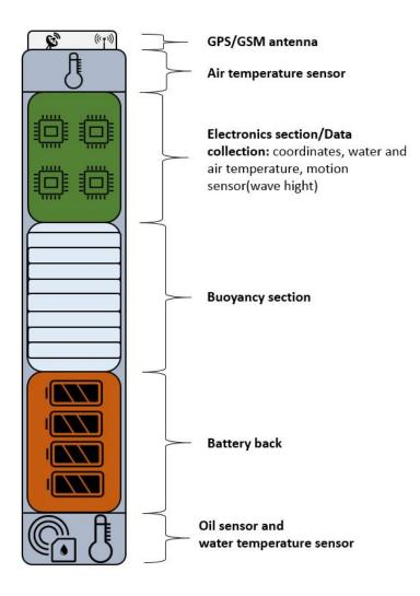
Figure 34 Rough schematics view of the oil detecting drifter buoy prototype.
